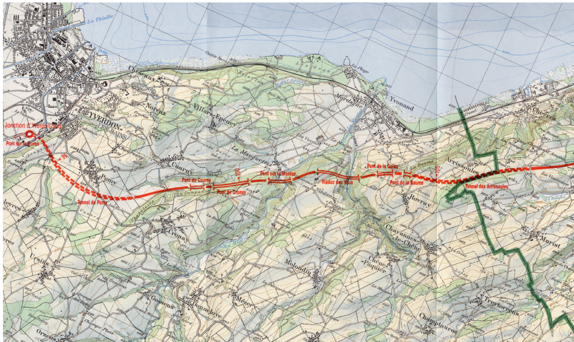
Figure 7.3 - Development of alternative routes for the highway A1 between Yverdon and Avenches in Switzerland. The original route alongside the lake, was relocated to the hinterland using a series of tunnels and viaducts. (Bundesamt für Strassenbau, Schweiz. Nationalstrassen N1. Reproduced by courtesy of the Federal Office of Topography, Berne, BA024489)
